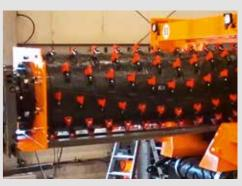
Exchange of shredding drum including bearing shield, No interference with power unit or gearbox.
